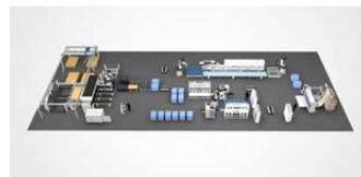
For medium-sized wood-processing businesses, we have developed processing cells that can be extended on a modular basis. Each individual cell is already an ideal solution for efficient panel processing. The individual cells are networked via a TRANSBOT, which is our name for the driverless transport robots.
